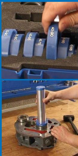
Select the correct collet size and sleeve using the chart above. The bearing must be at a right angle to the shaft. In addition, the shaft should be slightly lubricated.
